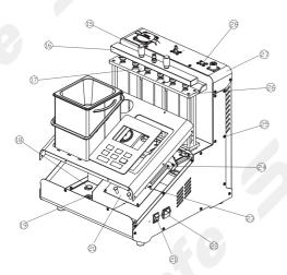
15-Compression Screw 16-Fuel Distributor 17-Adjusting Nut 18-Door Mat 19-Power Supply Base 20-Control Board 21-Power Switch 22-Power Socket&Fuse 23-Copper Pillar 24-Screw 25-Screw 26-Upper Pressing Plate 27-Cabinet 28-Copper Plug
