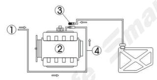
1-Injector Cleaner & Tester; 2-Engine; 3-stopper; 4- Fuel-inlet hose to engine;
